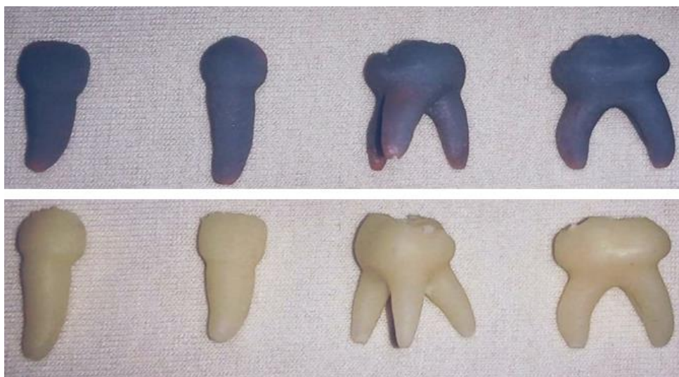
Figure 2. Teeth 51, 53, 54 and 84 printed in Anycubic Model resin (gray) and Bio Crown resin (white).
